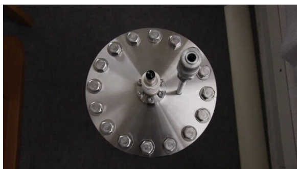
Figure 16. Stainless steel flange with electric power and gas connectors.
