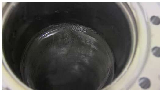
Figure 12. The stack of 3 nickel mesh reactants shown mounted in the reactor, unrolled against the reactor wall.
