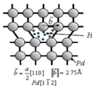
**FIGURE 1.** Scheme of edge dislocation loops in pd containing condensed h/d.
