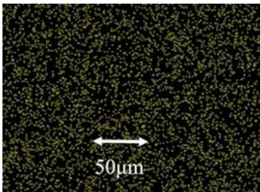
Figure 39. SEM photo of nitrogen distribution.
