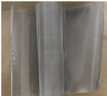
Figure 2. Nickel mesh as reactant, 30 cm<sup>2</sup>, 200 mesh. This photo shows the two meshes overlapped.
