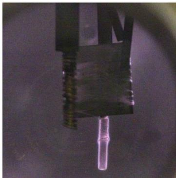
**Figure 6. Photo of plasma State when discharging by applying a high voltage to the Pd thin wire on the ceramic heater.**
