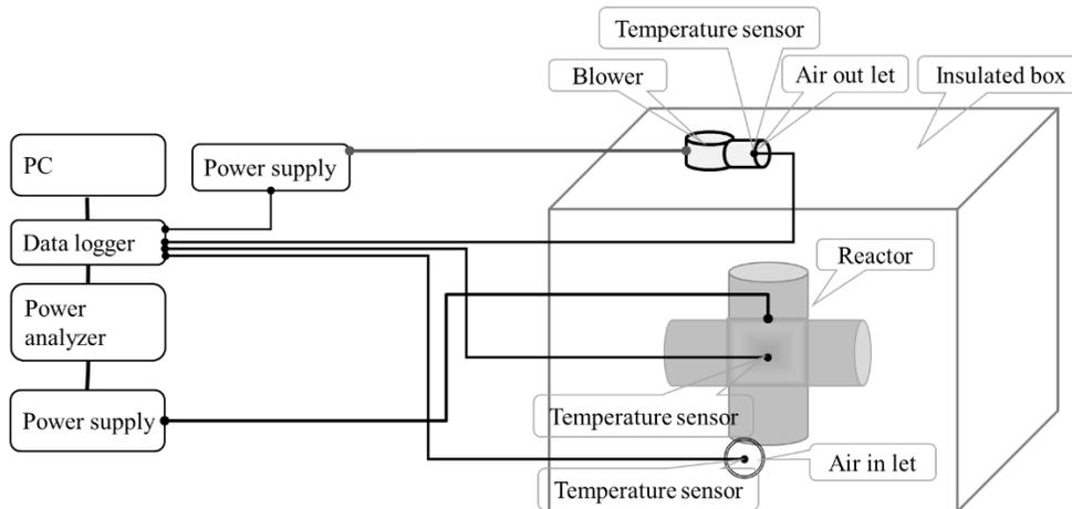
Figure 13. Schematic of measurement system
