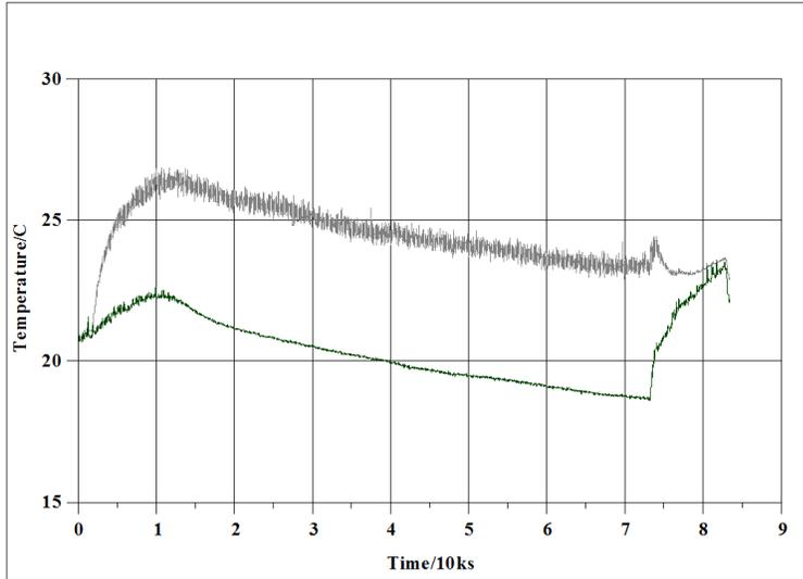
Figure 20. Temperature changes for inlet and outlet of the air at 100 W of input power before excess heat generation treatment.
