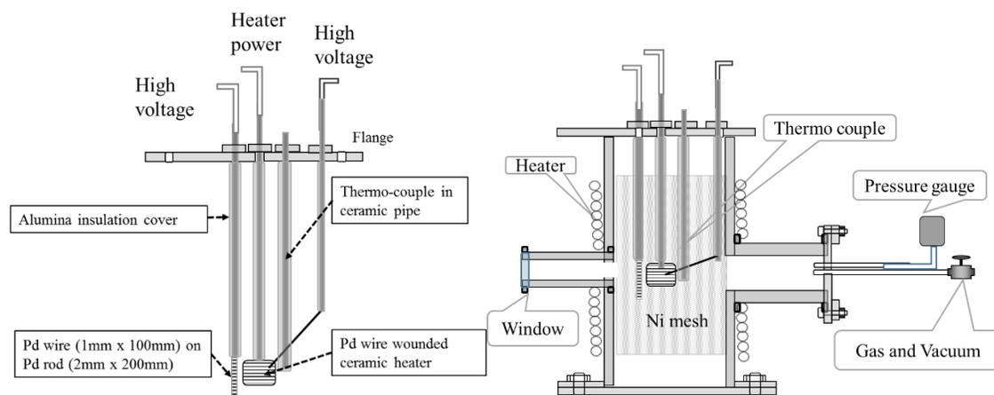
**Figure 4. Schematic representation of electrode and cross section of reactor.**
