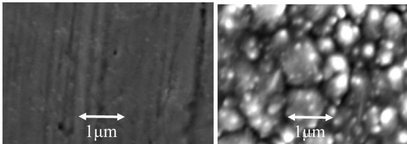
Figure 31. SEM photo of Ni reactant before treatment Figure 32. SEM photo of Ni reactant after treatment.
