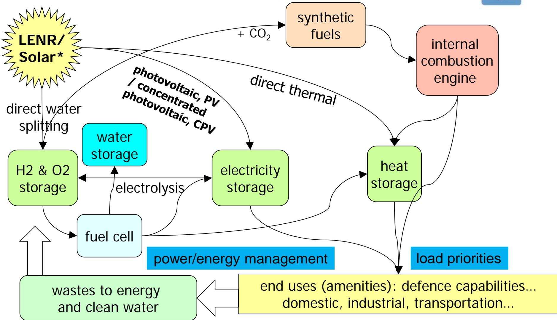
\* The LENR/solar energy source could be combined with (or replaced by) small hydro, wind and geothermal or new emerging energy technologies where available and suitable.
