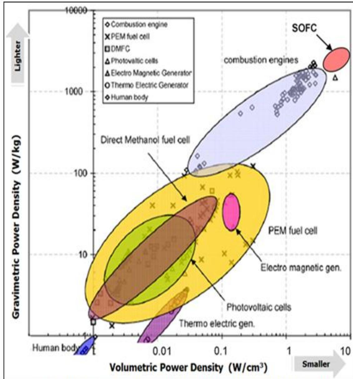
Legend: proton exchange membrane (PEM) fuel cell; and solid oxide fuel cell (SOFC).
