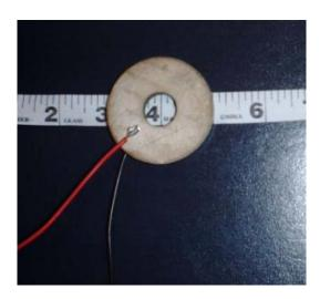
3" diameter 3/8" thick with a 1" hole in the middle
