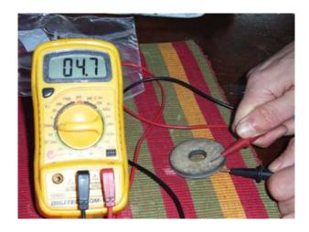
Polling is very hard to determine or measure. What Norm and Joel did was to clean the silver oxide from a small spot on each side of the piezo. Take your soldering iron and pre tin your leads leaving a bead of solder on the end of them. Carefully place the lead with the solder bead directly over the cleaned spot to where you are going to attach lead.
