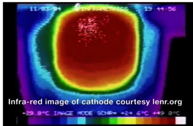
**Fig. 12.** (Color online) The images captured by the infrared camera in experiment of Stanislaw Shpak and others, 1994.
