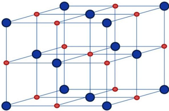
Fig. 2. (Color online) The crystal structure of  $fcc$  - palladium, platinum. Red circle denotes the deepest potential niches.
