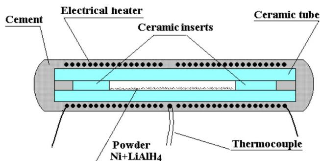
Fig. 13. (Color online) The scheme of A.G. Parkhomov's reactor.
