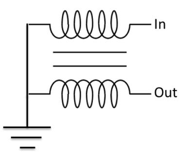
Primary consists of one wire looped many times around a single core – high inductance
